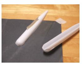
Use the edge of the hobby knife to scrape away the flashing around the seam. If the plastic gums up while scraping, the cement is not dry enough. Fill the seam voids with plastic model filler then sand and prime.
